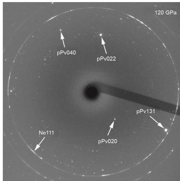
**Fig. 1.** A representative spotty powder XRD pattern of  $(\text{Mg,Fe})\text{SiO}_3$  pPv. The diffraction pattern was collected at a fixed  $\omega$  angle at 120 GPa after temperature quenching from 2400 K, showing the spottiness of the XRD pattern. Reproduced from Ref. [25] with permission of PNAS, © 2013. Ne: neon.
