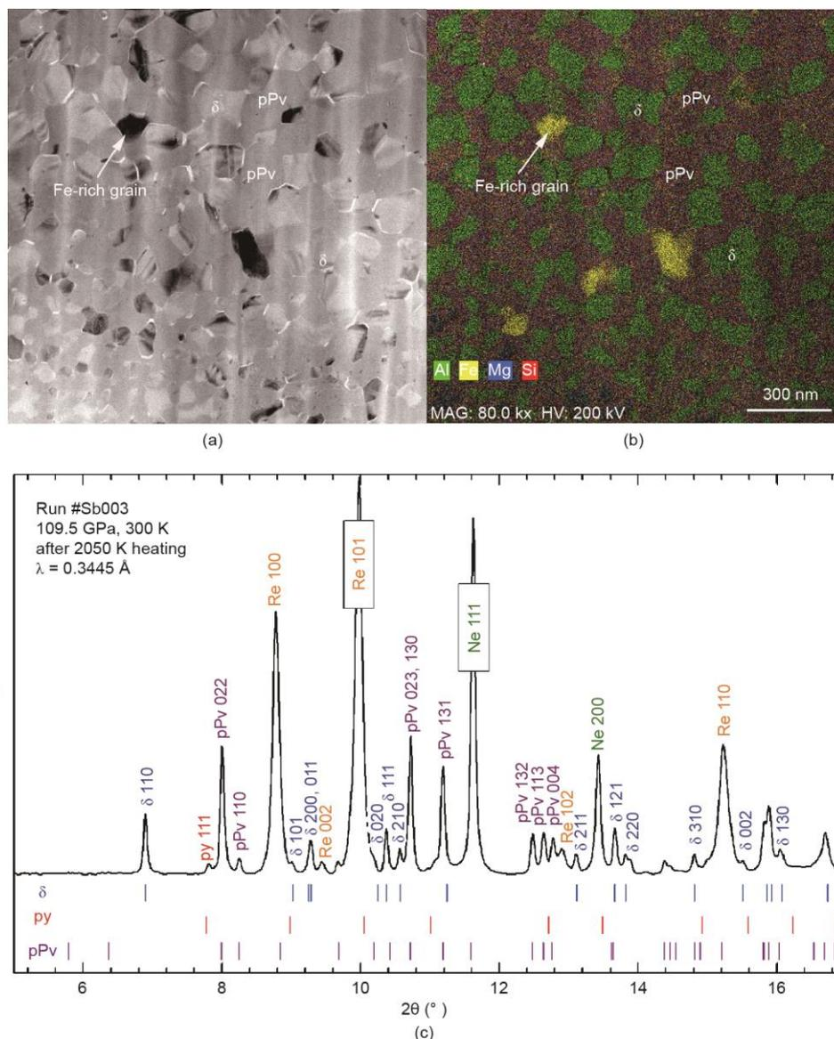
**Fig. 4.** A multiphase assemblage contains a dominant pPv phase, a hydrous  $\delta$ -phase, and a minor pyrite-type phase (py-phase) FeOOH. (a–b) TEM mapping shows a few Fe-rich grains, which is consistent with the existence of a minor py-phase suggested by (c) *in situ* XRD.
