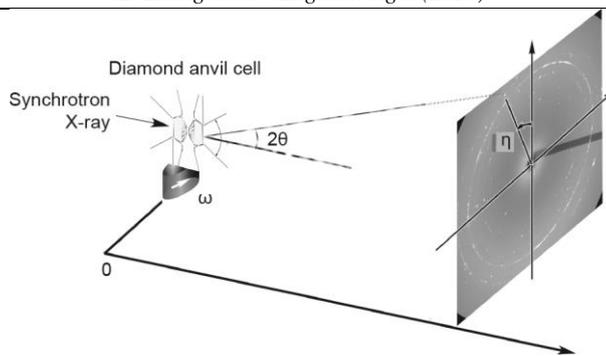
**Fig. 2.** Experimental setup for multigrain XRD data collection in a DAC. The sample is aligned to the rotation center, and a set of 2D XRD patterns are collected at small incremental steps, e.g.,  $0.2^\circ$ , to the angular access of a DAC, typically  $50\text{--}60^\circ$ , where  $\omega$ ,  $\eta$ , and  $\theta$  represent the rotation, azimuth, and Bragg angles of each reflection, respectively.
