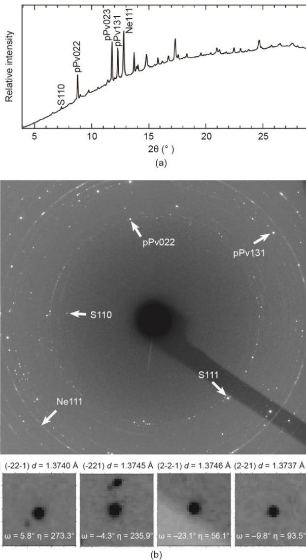
**Fig. 3.** XRD data of a phase assemblage including a dominant pPv phase and a minor phase of seifertite ( $\text{SiO}_2$ ). (a) An integrated powder XRD pattern showing the weak proportion of  $\text{SiO}_2$  at 129 GPa and after temperature quenching; (b) the multigrain XRD pattern including two Friedel pairs of  $\{221\}$  from one selected grain of seifertite. Reproduced from Ref. [30] with permission of GeoScienceWorld, © 2016. S: silica.
