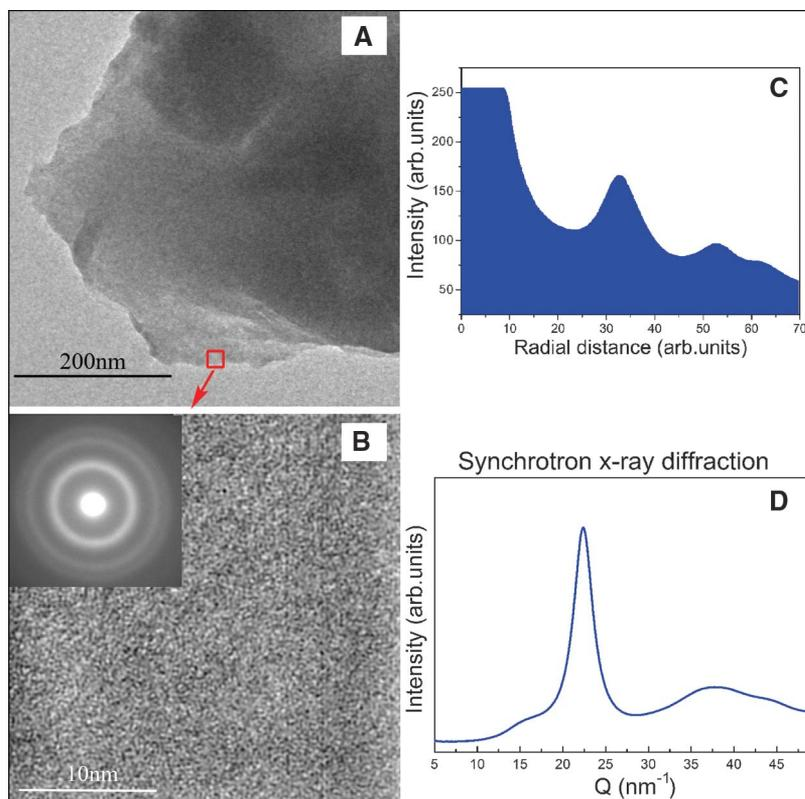
investigated and confirmed by HRTEM imaging, ED, and XRD analyses (Fig. 1). The MG ribbon was cut into specimens about 50  $\mu\text{m}$  by 40  $\mu\text{m}$  by 15  $\mu\text{m}$  in size. To ensure that we were looking at the internal bulk properties, all six surfaces of the rectangular specimen were recut or polished. A specimen was loaded in a diamond-anvil cell (DAC) along with ruby as the pressure calibrant and helium as the hydrostatic pressure-transmitting me-
