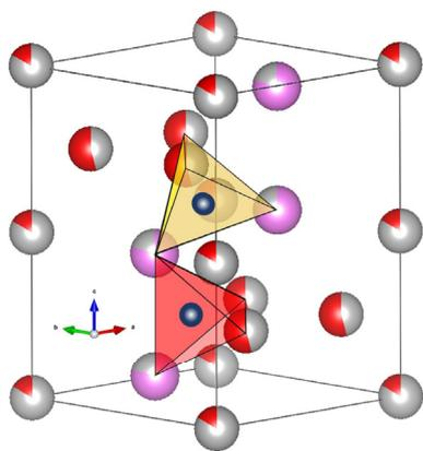
**Fig. 3.** Structure modeling of as-cast  $\text{Ti}_{53}\text{Zr}_{27}\text{Ni}_{20}$  C-14 Laves phase with deuterium positions is illustrated by using VESTA. Ti, Zr, Ni and D are represented in grey, pink, red, and blue, respectively. The fraction of the color of the atom represents the occupancy of the shared site. The tetrahedrons are indicated with solid lines. (For interpretation of the references to color in this figure legend, the reader is referred to the Web version of this article.)
