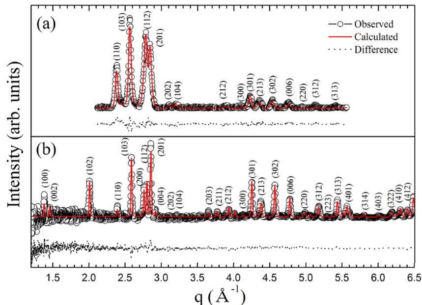
**Fig. 1.** Results of Rietveld refinements for (a) X-ray and (b) neutron diffraction patterns measured from as-cast  $\text{Ti}_{53}\text{Zr}_{27}\text{Ni}_{20}$  alloys. The diffraction data and calculated peaks for C14 phase are shown with circles and solid lines, respectively. The difference between the data and simulation is shown in dots.
