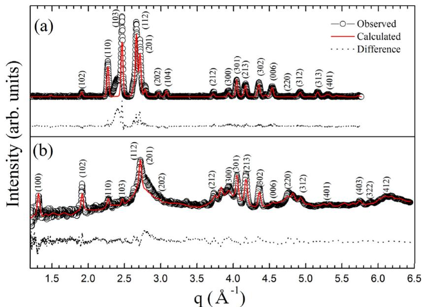
**Fig. 2.** Results of Rietveld refinements for (a) X-ray and (b) neutron diffraction patterns measured from partially deuterated  $\text{Ti}_{53}\text{Zr}_{27}\text{Ni}_{20}$  alloys. The diffraction data and calculated peaks for C14 phase are shown with circles and solid lines, respectively. The difference between the data and simulation is shown in dots.
