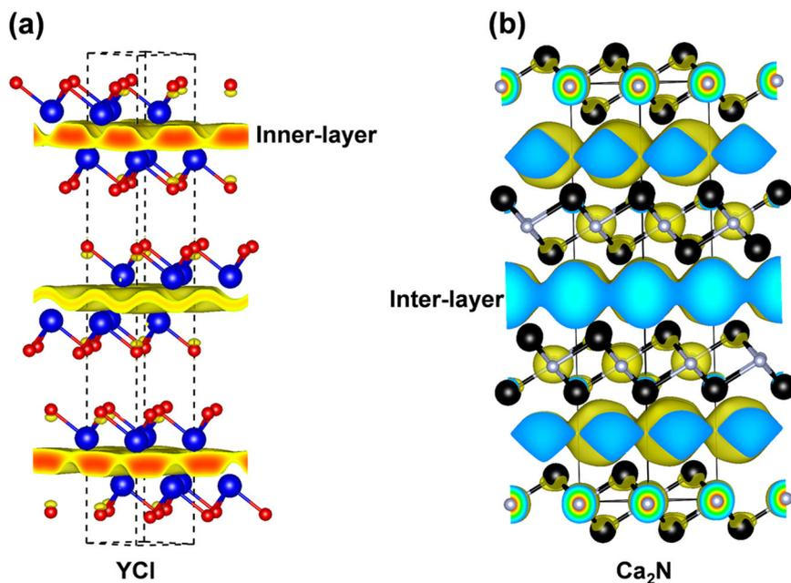
**Fig. 5** Charge density of interstitial electrons in (a) YCl and (b) Ca<sub>2</sub>N, the white and black spheres in Ca<sub>2</sub>N represent N and Ca atoms, respectively
