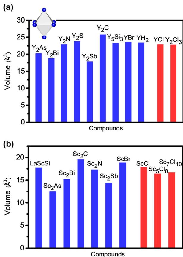
**Fig. 2** Interstitial volumes of  $R_6$  octahedron in YCl,  $Y_2Cl_3$ , ScCl,  $Sc_5Cl_8$ , and  $Sc_7Cl_{10}$ , comparing with other (a) Y and (b) Sc contained electrides. Interstitial volumes of  $R_6X$  octahedron in Cu<sub>2</sub>Sb-type compounds:  $Sc_2As$ ,  $Sc_2Sb$ ,  $Sc_2Bi$ ,  $Y_2Sb$ , and  $Y_2Bi$  were also collected
