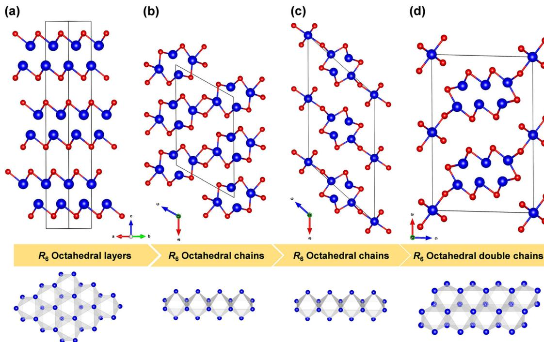
**Fig. 1** Crystal structures of (a) YCl, (b)  $Y_2Cl_3$ , (c)  $Sc_5Cl_8$ , and (d)  $Sc_7Cl_{10}$ . The blue and red spheres represent the Y/Sc and Cl atoms, respectively. The edge-sharing  $R_6$  octahedra in the host structures condensed into edge-sharing layers, chains and double chains, which are displayed at the bottom
