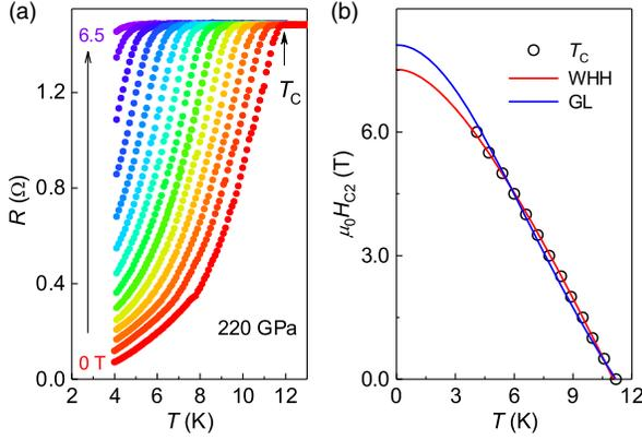
FIG. 2. The determination of zero-temperature upper critical magnetic field  $\mu_0 H_{c2}(0)$  of  $2H_a$ -MoS<sub>2</sub> at 220 GPa. (a)  $R$ - $T$  curves under external magnetic fields of up to 6.5 T at steps of 0.5 T. (b)  $\mu_0 H_{c2}$ - $T$  phase diagram. The solid line in red and blue represents fitting by the WHH formula and GL equation, respectively.
