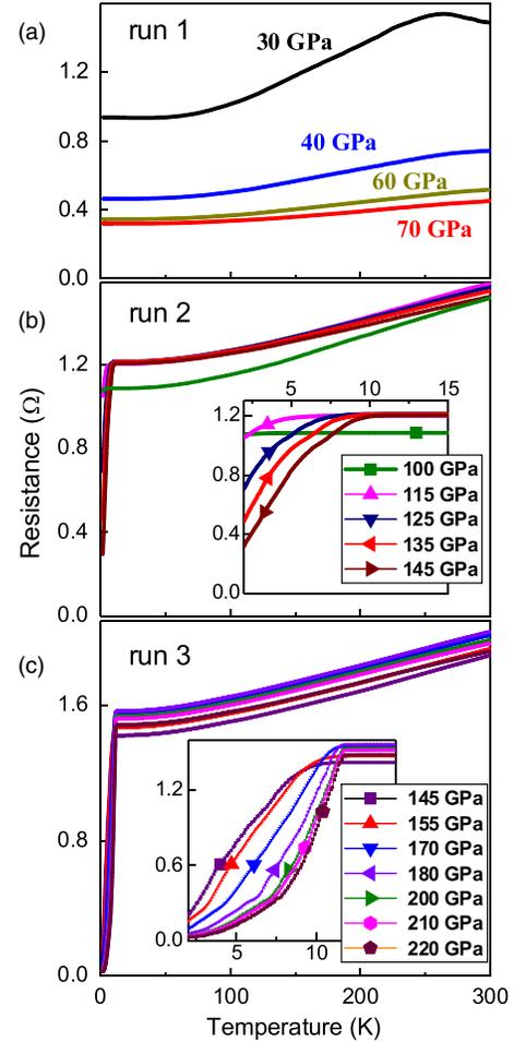
FIG. 1. Temperature-dependent resistance of  $2H_a$ -MoS<sub>2</sub> at elevated pressures. (a)  $R$ - $T$  curves at pressures between 30 and 70 GPa in run 1. (b)  $R$ - $T$  curves at pressures between 100 and 145 GPa in run 2. (c)  $R$ - $T$  curves at pressures between 145 and 220 GPa in run 3. The inset in (b) and (c) is the close-up of the low-temperature region, highlighting the superconducting transition.
