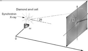
Fig. 2. Experimental setup for multigrain XRD data collection in a DAC. The sample is aligned to the rotation center, and a set of 2D XRD patterns are collected at small incremental steps, e.g.,  $0.2^{\circ}$ , to the angular access of a DAC, typically  $50-60^{\circ}$ , where  $\omega$ ,  $\eta$ , and  $\theta$  represent the rotation, azimuth, and Bragg angles of each reflection, respectively.
