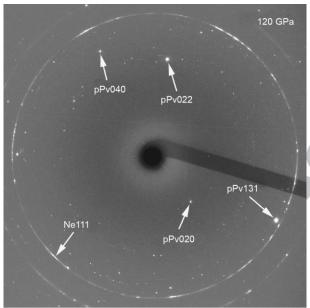
Fig. 1. A representative spotty powder XRD pattern of (Mg,Fe)SiO<sub>3</sub> pPv. The diffraction pattern was collected at a fixed ω angle at 120 GPa after temperature quenching from 2400 K, showing the spottiness of the XRD pattern. Reproduced from Ref. [25] with permission of PNAS, © 2013. Ne: neon.
