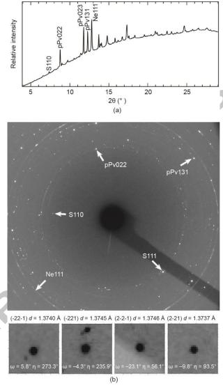
Fig. 3. XRD data of a phase assemblage including a dominant pPv phase and a minor phase of seifertite (SiO<sub>2</sub>). (a) An integrated powder XRD pattern showing the weak proportion of SiO<sub>2</sub> at 129 GPa and after temperature quenching; (b) the multigrain XRD pattern including two Friedel pairs of {221} from one selected grain of seifertite. Reproduced from Ref. [30] with permission of GeoScienceWorld, © 2016. S: silica.
