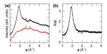
FIG. 1. Background correction of integrated diffraction patterns. (a) Diffraction pattern of fluid CH<sub>4</sub> at 0.69 GPa (black, upper) and background from empty DAC (red, lower). (b) Static structure factor S(q) of CH<sub>4</sub> at 0.69 GPa obtained by subtracting background and normalizing in the high-q limit.
