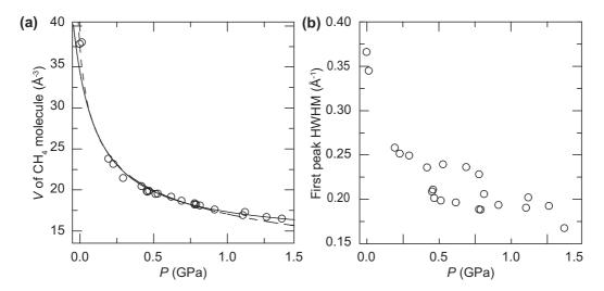
FIG. 2. (a) Equation of state (EOS) of fluid CH<sub>4</sub> at 298 K. Circles: experimental data. Solid line: Fit of ideal gas EOS modified with van der Waals correction [Eq. (4)]. Dotted line: Fit of Murnaghan EOS [Eq. (1)]. (b) HWHM of first peak in S(q) plotted as a function of pressure at 298 K.
