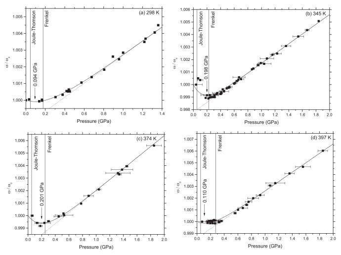
FIG. 3. Plot of reduced frequency of CH<sub>4</sub> Raman-active vibration as a function of pressure at (a) 298 K, (b) 345 K, (c) 374 K, and (d) 397 K. Solid lines following the data are fits performed using Eq. (6) and arrows signify the minimum of this fit. Dotted lines are linear fits to data collected above 0.6 GPa [Eq. (5)]. Vertical solid lines are expected positions of the Joule-Thomson line and Frenkel line.
