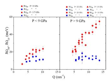
Figure 2. Dispersion curves below and above the PA crossover. Best-fit dispersion of  $\Omega_{\rm LF}$  (blue symbols) and  $\Omega_{\rm HF}$  (red symbols) as measured at the indicated pressures below (left panel) and above (right panel) the PA transition.
