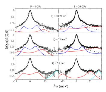
**Figure 1. IXS spectra below and above the PA crossover.** Representative IXS spectra of v-GeO<sub>2</sub> measured at low and high pressures for selected *Q* values (open circles). The thick black line corresponds to the best-fit model line-shape in Eq. 1, with its low frequency (blue line) and high frequency (red line) DHO components. The dashed and cyan lines represent respectively the resolution function and a DHO profile accounting for the transverse mode of the diamond anvils.
