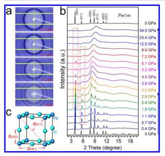
**Figure 1.** Synchrotron XRD patterns of MAPbBr<sub>3</sub> obtained during compression up to 34.0 GPa and decompression: (a) The raw 2D XRD images and (b) integrated 1D XRD profiles. The XRD pattern after decompression can be indexed with the same crystal structure (space group  $Pm\overline{3}m$ ) from the pristine materials. (c) Illustration of the representative interplanar distances in MAPbBr<sub>3</sub> lattice (Only Pb and Br atoms are drawn for clarity).
