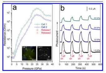
**Figure 6.** Electrical resistance (a) and photocurrent (b) of  $MAPbBr_3$  as a function of pressure. The insert in panel (a) displays microphotographs of the samples in two DACs with Au probes.
