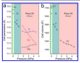
**Figure 3.** Unit cell parameters (a) and volume evolutions (b) of MAPbBr<sub>3</sub> as a function of pressure at room temperature. Space group of I: cubic,  $Pm\overline{3}m$ ; II: cubic,  $Im\overline{3}$ ; III: orthorhombic, Pnma.
