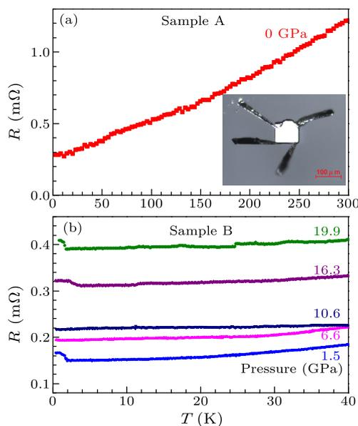
**Fig. 2.** The resistance of NbAs single crystal under various pressures. (a) The value of  $R(T)$  of sample A measured at ambient pressure. (b) The value of  $R(T)$  of sample B measured under pressures up to 20 GPa. Inset: the typical configuration of resistance measurement for NbAs single crystal. Four Pt electrodes were attached to the sample corners with silver epoxy.
