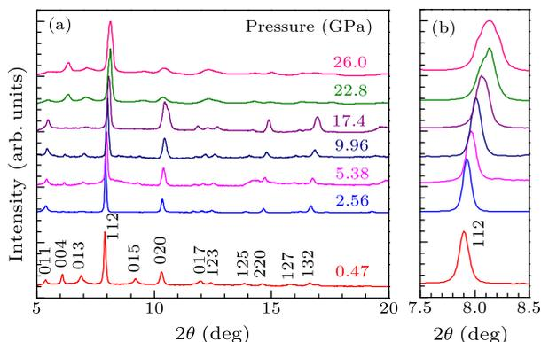
**Fig. 1.** In-situ powder synchrotron XRD patterns of NbAs under various pressures up to 26 GPa at room temperature, with the x-ray wavelength  $\lambda = 0.3100 \text{ \AA}$ . (b) Pressure evolution of the (112) peak. The shift towards higher angle indicates the shrink of the lattice under pressure.
