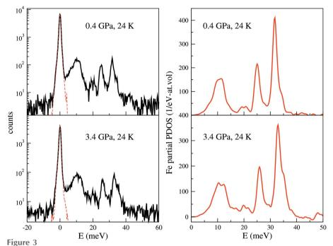
(Left) NRIXS spectra of  $Eu^{57}Fe_2As_2$  under high pressures and 24 K (solid lines) and instrumental resolution function (red dashed lines) measured by SMS. The intensity of the resolution function is scaled to the elastic peak intensity in the NRIXS spectra. (Right) Derived Fe specific PDOS.
