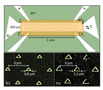
FIG. 1. (Color online) Upper panel: sketch of the transport bridge with the corresponding dimensions. Lower panels: scanning electron microscopy images of the Al samples with the triangular array of triangular antidots.
